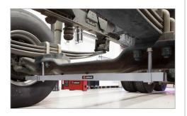
An uneven floor will influence measurements of angles like camber, caster and KPI. By use of the inclinometer kit the cam-aligner system will automatically compensate for all these effects.
