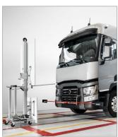
Radar & camera calibration requires the Volvo Group Wheel Alignment system and JOSAM cam-aligner software (version 1.7.4 or higher).
